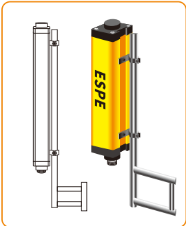
Rotary arm reinforced installation method
